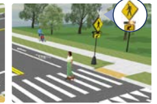
Rectangular Rapid Flash Beacons use flashing lights to warn drivers of pedestrians crossing, enhancing safety at unsignalized crossings.
