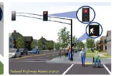
Signalized Intersection Enhancements improve pedestrian safety by adding features like countdown signals, and leading pedestrian intervals.
