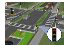
Bicycle Signals and Conflict Zone Markings increase bike lane visibility and reduce collision risks at intersections.
