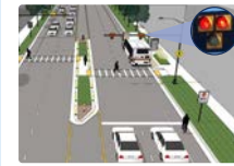
Pedestrian Hybrid Beacons alert drivers to stop for pedestrians, improving safety at crossings without traditional traffic signals.
