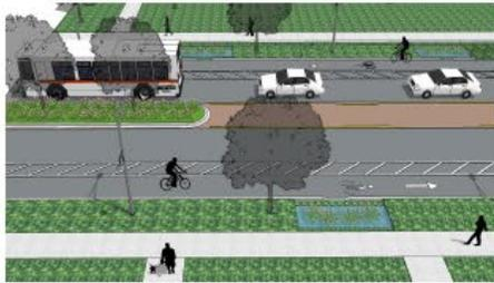
Where space permits, a painted buffer zone should be incorporated between the bike lane and the motor vehicle lane for added safety and separation from vehicles. Flexible posts may also be included as to increase bicyclists comfort.
