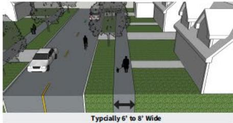
To ensure a more user-friendly and accommodating experience for all, bicycle and pedestrian facilities should be separated. In areas with higher bicycle use or where separated bicycle facilities are not provided, a sidepath should be included.
