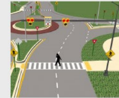
Roundabout with Pedestrian Hybrid Beacon
