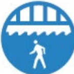
Optional: 24-inch diameter stencil or 12-inch sticker with pedestrian symbol
