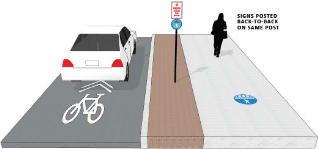
Optional: 24-inch diameter stencil or 12-inch sticker with pedestrian symbol
