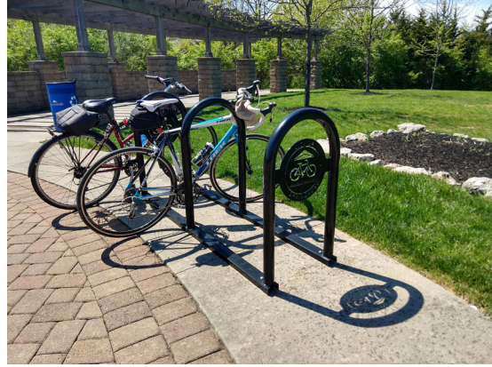
The bicycle racks should be placed and spaced in compliance with the APBP Bicycle Parking Design Guidelines where any part of a parked bicycle is at least two feet back from the edge of the trail.
