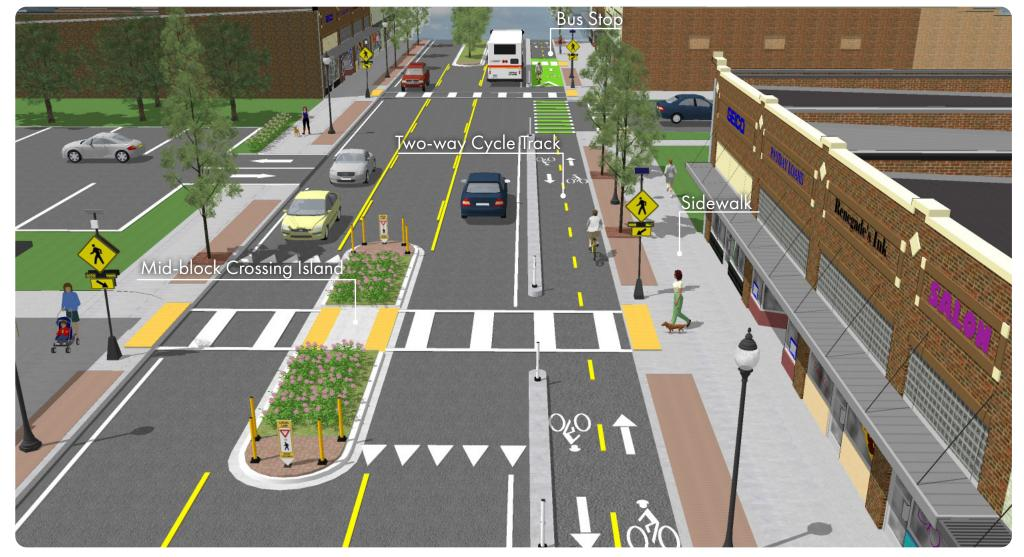
Where space is limited, the two-way cycle track will be separated from the motor vehicle traffic by a raised divider.
