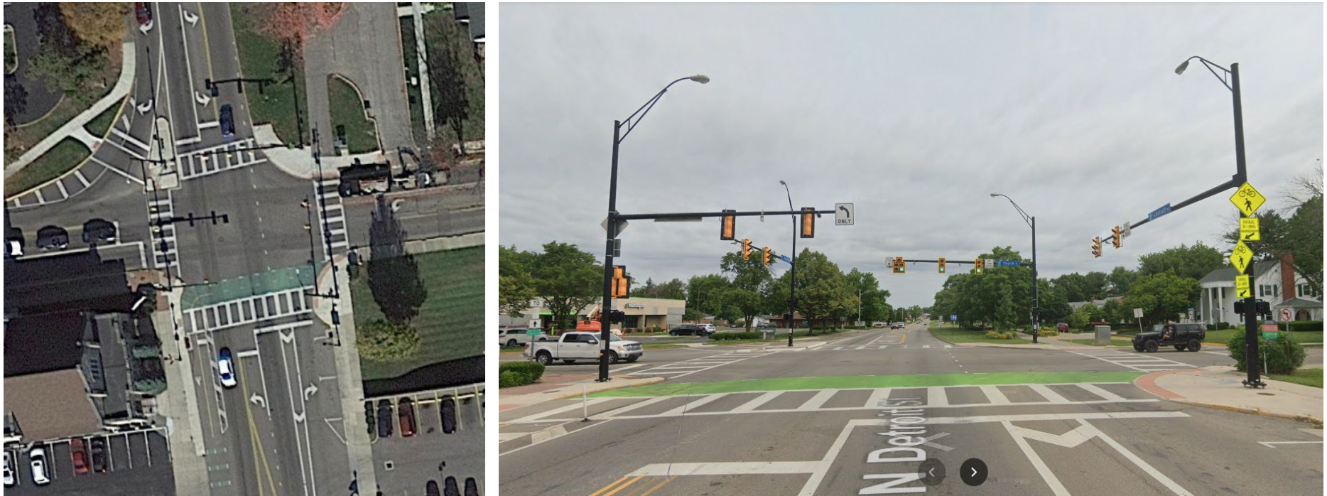
Figure 30: Transition from two-way cycle track to sidepath in Xenia, OH (Source: Google Maps)
